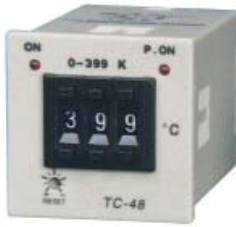
TC-48 Coding setting, number indication thermoregulator Outer dimension: 48x48x96mm Hole dimension: 45x45mm
