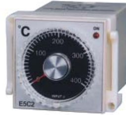
E5C2 Dial setting, no indicating thermoregulator Outer dimension: 48x48x96mm Hole dimension: 45x45mm
